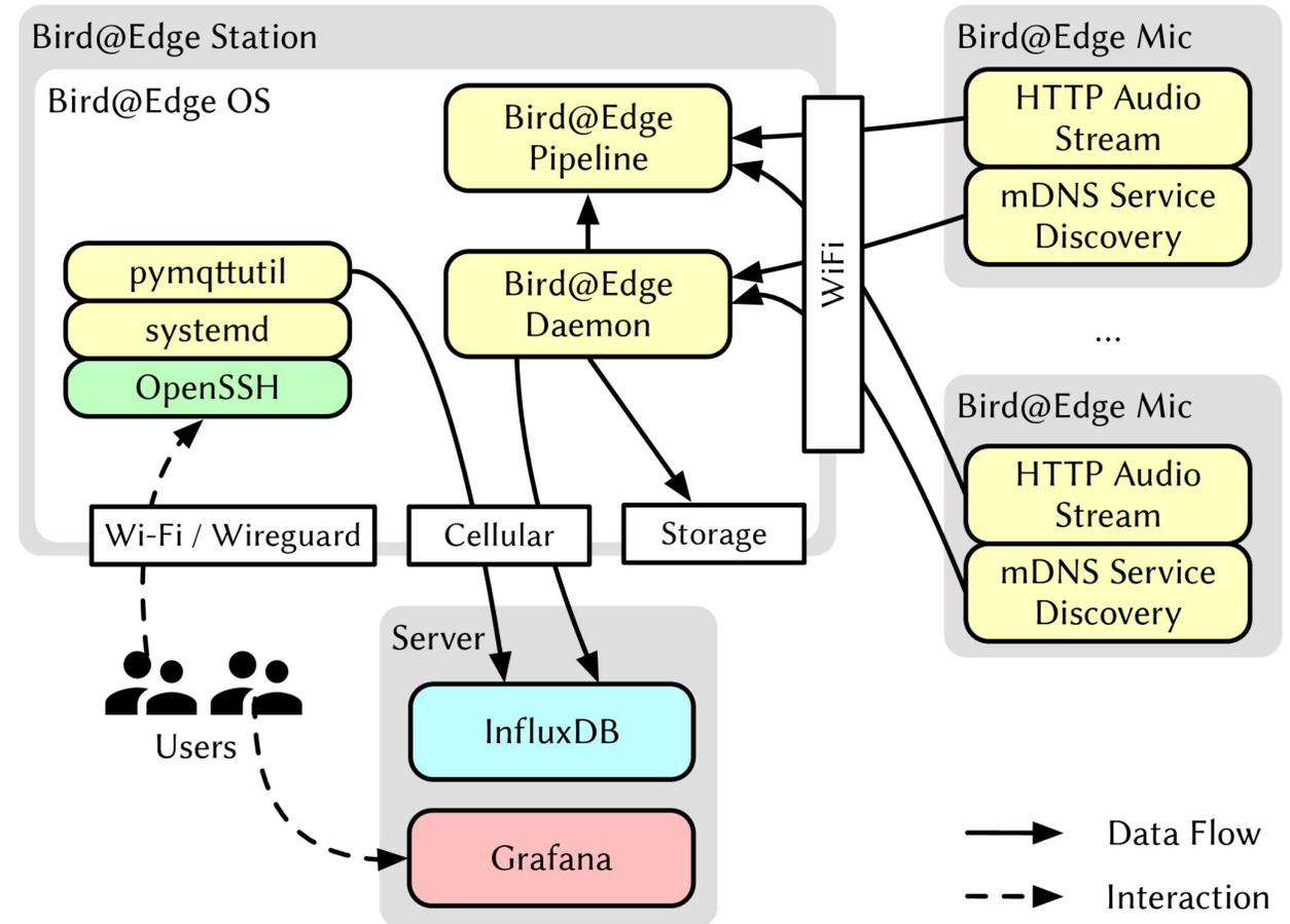
Fig. 3: Bird@Edge software components
