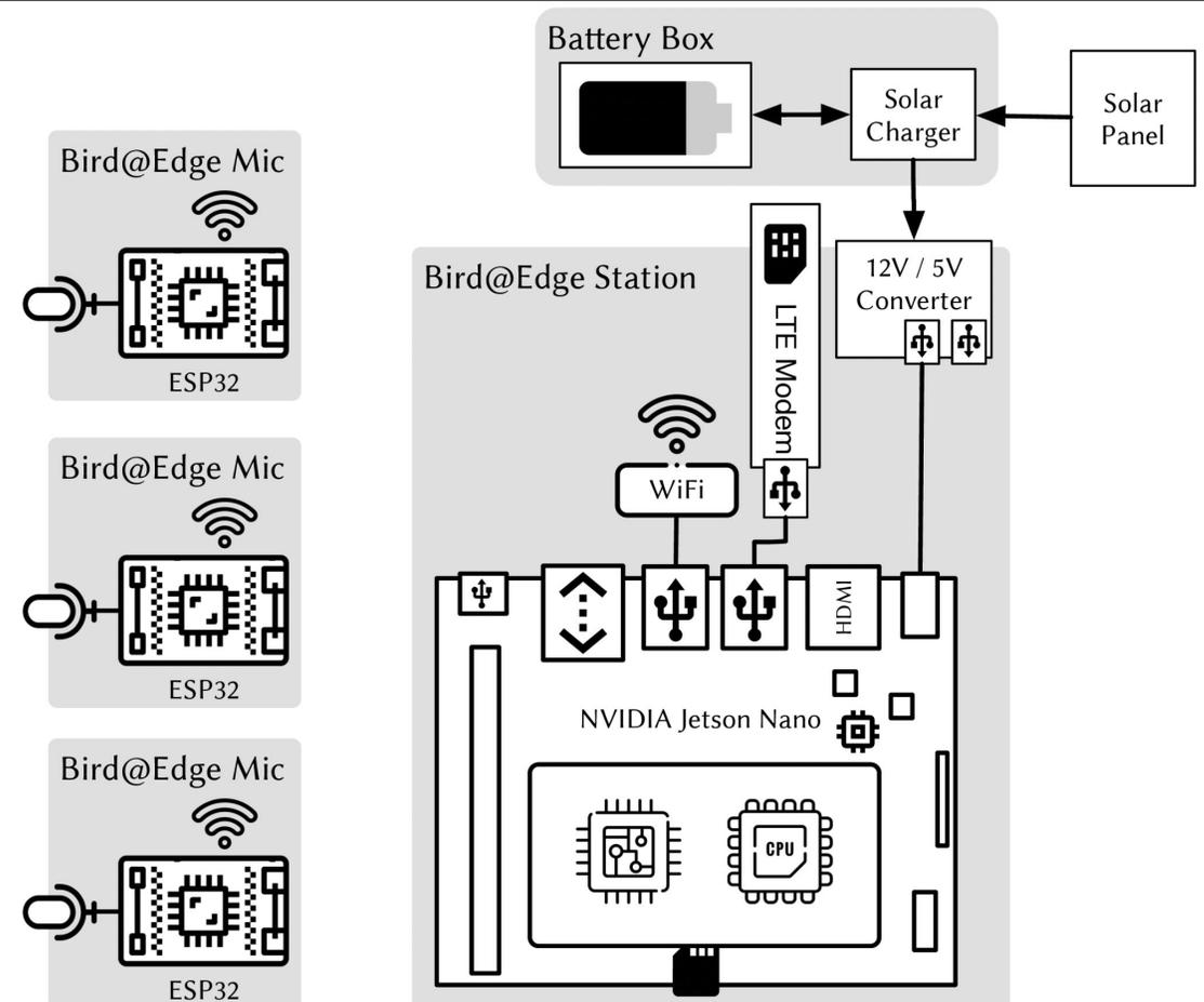
Fig. 2: Bird@Edge hardware components
