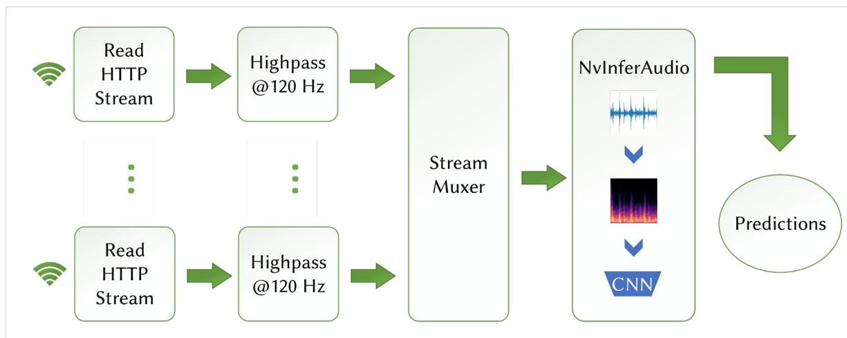
Fig. 4: Overview of the Bird@Edge processing pipeline
