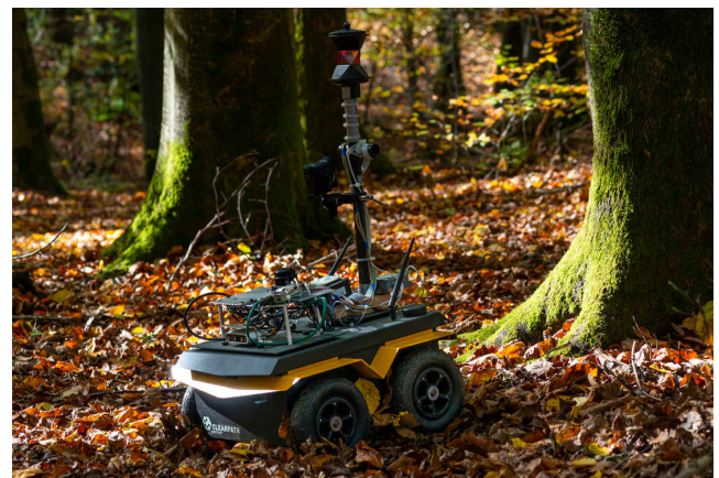
FIGURE 13 Multisensor rover platform. Rover equipped with multiple sensors and a prism for tracking by a robotic total station. Photo: M. Dobbermann.
